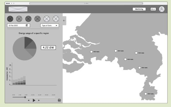
Opened menu - has a timeline slider to select different timeframes. The user can enable and disable different energy sources. The user can view information about the selected grid.
